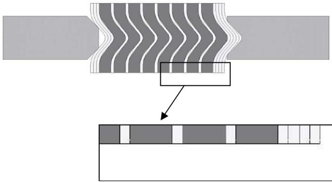
FIGURE 25: FILLER FLUSH WITH WINDING METAL
