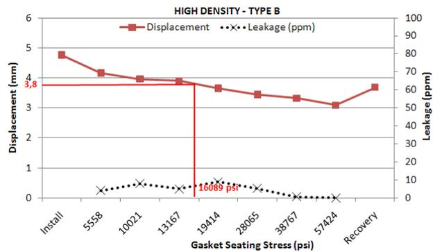
FIGURE 24: HIGH DENSITY STRESS X DISPLACEMENT
