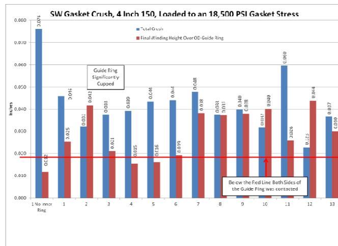
FIGURE 33: SW Winding Crush
