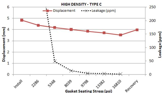
FIGURE 32: HIGH DENSITY – TYPE C
