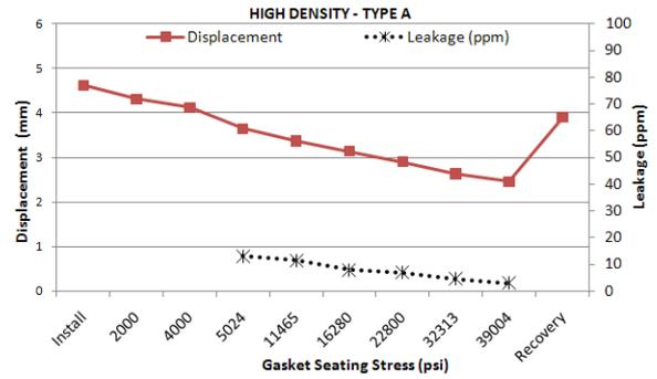
**FIGURE 12: HIGH DENSITY – TYPE A**
