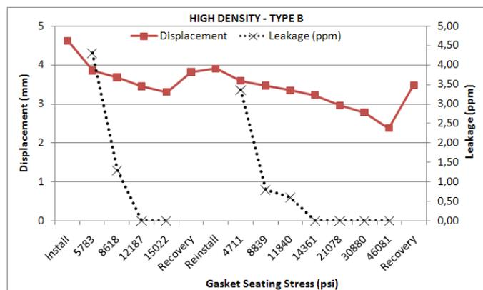
FIGURE 34: SW Gasket Sealability after Reinstallation
