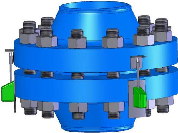
**FIGURE 7: GASKET DISPLACEMENT TRANSDUCERS**
