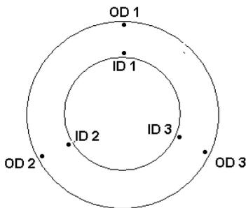
FIGURE 17: WINDING THICKNESS LOCATIONS
